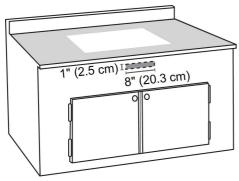
3 Cut a  $20 \times 1.2$  in. (50.8  $\times$  3.0 cm) hole into the back wall of your cupboard to vent your cooktop. Make sure that the cut is centered and 1 in. (2.5 cm) from the surface of your counter.
